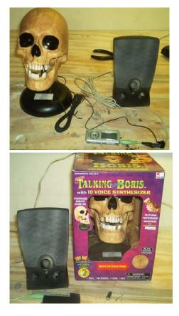
Here is everything you need for this project; A 100 microfarad capacitor, a 10 ohm resistor, a powered computer speaker, and a Boris. You will also need a music source you can plug the speaker into for testing
