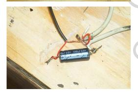
Finally twist the bare copper wire from the Boris around the bare copper wire from the speaker, and solder this. Plug the speaker back in, and turn Boris on. You should be able to turn up the sound and the Boris will start talking. You should be able to hear sound from both the computer speaker and the Boris speaker. Unplug the speaker.
