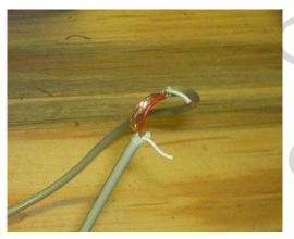
Carefully strip 1-2 inches of the outer insulation from the speaker cord, about 6 inches back from the 3.5mm phone plug (also called a TRS). I use strippers to barely cut through the outer insulation, then I pull the necessary cover away with my finger nails. If this does not work you can use needle nose pliers to pull the insulation back, or a pair of diagonal cutters or small scissors to cut away the cover. Be careful not to cut the wires inside the cover.
