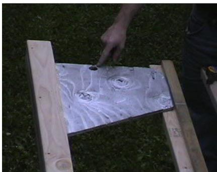
Next, cut your blade. Mine is about 15" wide and you can use the entire length of the board if you want. Start from the lower corner and make a cut at an angle to about halfway up on the other side. Take a C clamp and clamp it to the top. You want to find the center of gravity to make the edges plumb. Mark your hole where the clamp is. This will look off center. That's OK, its supposed to.
