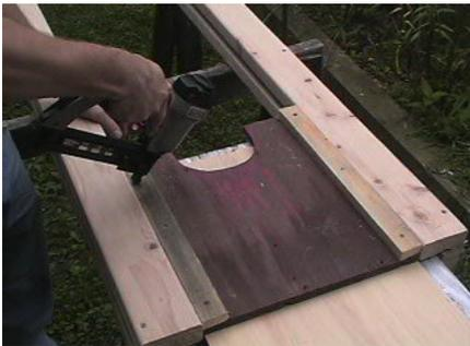
Now, slide the blade to the bottom end. You will need to cut two matching pieces of 1/2" plywood to fit between the side rails. Don't forget to cut out the area that the neck will lay in. While the blade is in the groove, lay a 1/4" spacer between the blade and the plywood you just cut and fit it into place. This will allow enough space for the blade to glide down the guillotine freely.
