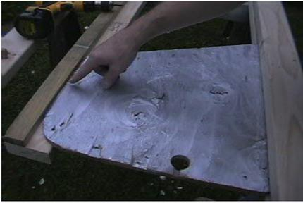
Take the new blade and slide it into the grooves and make certain there aren't any tight spots. Then move the blade to the top. Cut a piece of 2" furring strip and square it across the top. This provides a place to attach a pulley. Double-check that your blade moves freely and screw the top in place.
