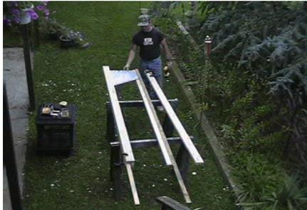
Make sure you have saw horses or something similar to work on. First, take two 2x4x8's and sandwich a 5/8x2x8 in between. Keep all three pieces flush to one side and close together. Fasten both sides with 2 and a half inch screws. I like to pre-drill the holes first as it makes things a lot easier.
