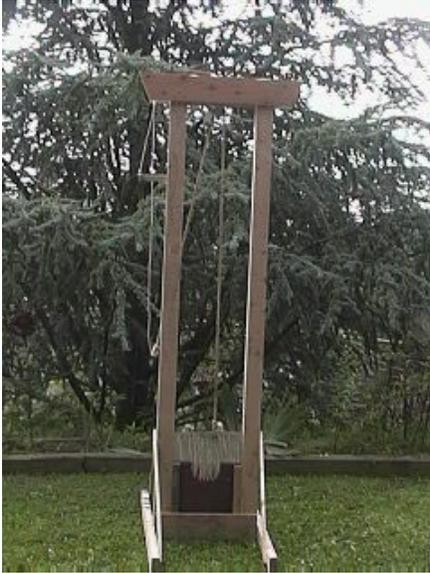
Leave enough room for the pulley plus 4" between the top of the blade and frame. When you have the blade where you want it, find the upper angle of the cutting edge. This will be the center mark of the hole you are going to make in the side of the blade track. Length of hole is about 4-1/2".
