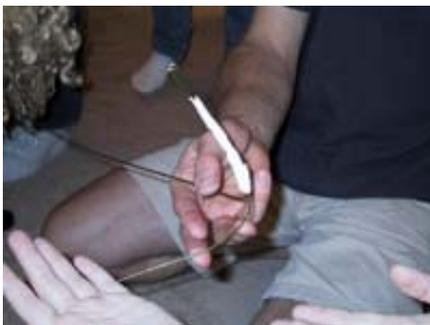
We taped two wire ends together. The wire has a bend at the top. This 'hook' catches back into the head so the wire doesn't pop out.
