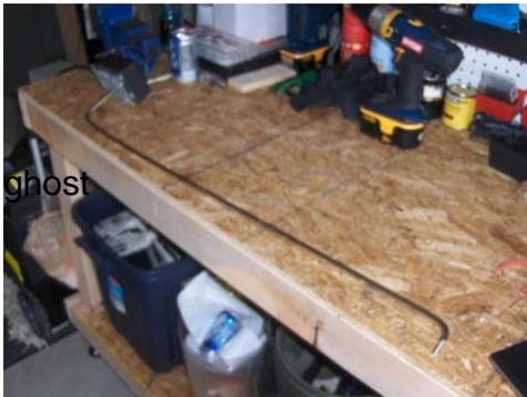
Bend shaft 90 degrees at motor and at other end. The rotisserie shaft is also too long so you will need to cut it off to your desired length. That will be determined by the size of your
