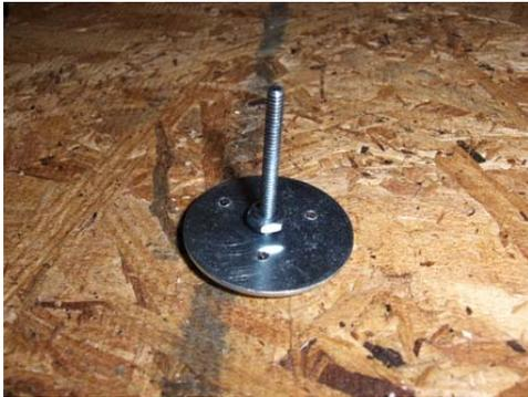
Install bolt and nuts so washer spins freely.
