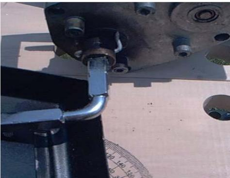
This is another pic of the nail through the driveshaft of the motor.
