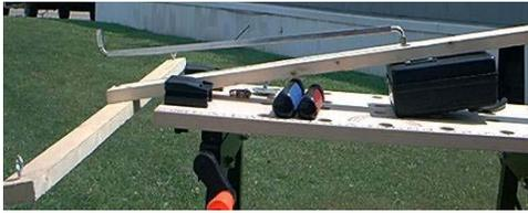
This is the motor all back together with the crank attached. I fed the crank through a 5/8" hole in the platform. Note the shape of the crank. I bent the square rod by putting it in a crack in the sidewalk and leaning on it!!! It works. Also note the eyelets that the fishing line will run through. There is one on each corner of the platform.
