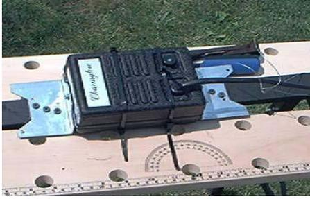
This is the steel bracket I mounted on the end of the motor to keep it from slipping around. The bracket was found at the lumberyard among the truss plates. Don't know exactly what this thing is called but it works great for this. I had to drill a hole to match up with the screw on the motor and for the three drywall screws I fastened it to the platform with. I put one of these brackets on each end of the motor. They keep the motor very still and no twisting occurs while its running.
