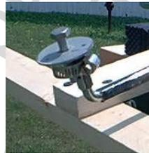
These are pics of the spool that goes on the end of the crank. Its nothing more than a large fender washer with three holes drilled in it on a large bolt. I can't tell you what size the bolt is but about any size will do. I ran the nut on the bolt down until it was out of threads. A little hose clamp was used to fasten the spool to the end of the crank.
