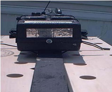
I then lined up the motor on top of the platform. Then I temporarily fastened the motor to the platform with black wire ties. Note the little silver screw about 1/2 way up on the end of the motor. I used it to fasten a steel bracket to keep the motor from shifting around while the crank was rotating.
