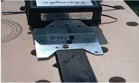
Here is a pic of both brackets fastened on to the motor. I left the wire ties on there. Couldn't hurt anything. You may have to use something else to keep your motor from twisting around but for this particular one these brackets work great.
