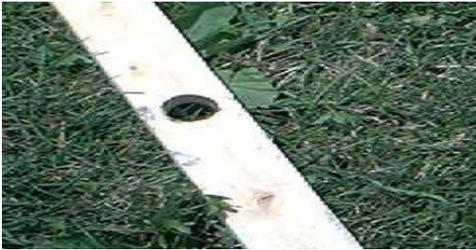
This is the hole through the platform for the shaft of the motor and the crank. The hole was drilled with a 5/8" spade bit. I drilled about 1/2 way through the 1X2 with the bit and then flipped it over and drilled the rest of the way through to prevent splintering.
