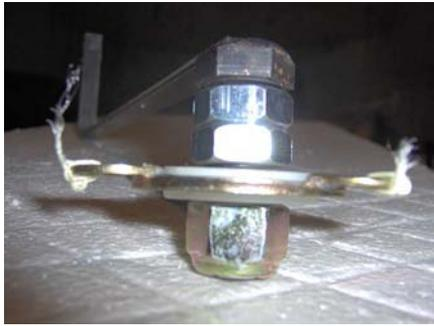
I then attached the crank arm to the motor shaft using a wire clamp connector I found at the hardware store. The regular u-bolt recommended by the other sites wouldn't work for me. At first I couldn't find them at the hardware store, and when I did, none of the sizes seemed to be appropriate. The one I used did the job, but it did come apart a couple of times. Mainly due to not being tightened
