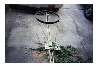
This is the drive unit. It gets mounted onto another strut in the tree in a pivoting fashion. This 'scissors' action allows a simple bungee cord to act as a tensioner.
