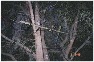
Here's a shot of the drive unit all mounted and strung with a test line. Note the bungee tensioning rig. I used the flourescent line to keep from hanging the ladder (and my throat) in it while I set it up
