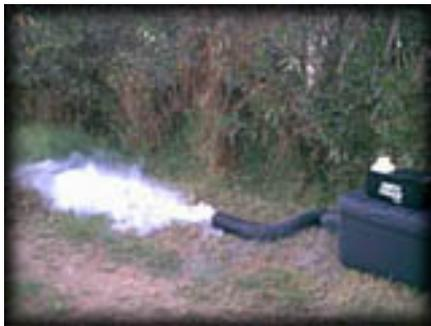
Yes, fog can easily go through large Shop-Vac type hose for about 6 to 8 feet, but after that you'll need a small fan to help push the fog through the hose. Smooth hose works better than corrugated. You should never attach the hose directly to the fogger, an inch or so of space between the hose and fogger is safer and will give you better fog distribution. This works great when attached to a Fog Chiller as show to the right.
