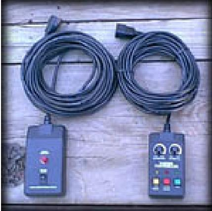
All fog machines come with some type of activation device, usually in the form of a simply remote control connected to the fog machine via a long cable. To start making fog you hold down the button on the remote. When you let up on the button it will stop making fog or it will stop automatically when the fog machine needs to re-cycle. The problem with this type of remote is that it requires a user to operate it every time you want more fog.
