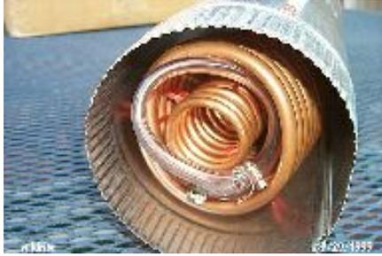
Now, connect the inner and outer coil with a short piece of plastic tubing and pipe clamps.
