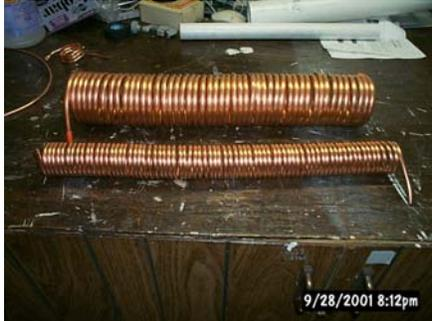
Once the coils were made, I pulled the scrap PVC out of them and spread them apart a bit like a spring till they were the same length as the stove pipe.
