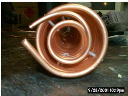
Now slide the smaller coil into the bigger coil. (see below)
