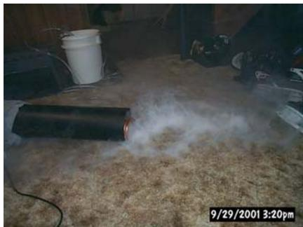
Here you can see that I used a rag or shirt to clog up the end with the fog machine to make sure ALL the fog goes through the chiller. (some was sneaking out the same side un-chilled) Notice also my bucket of ice and the lines running to it.
