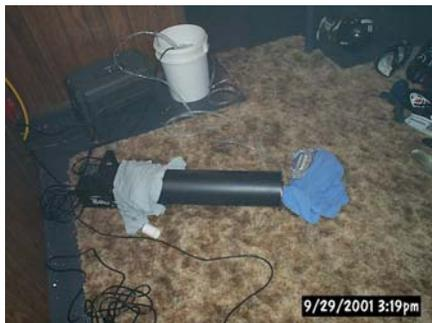
Here you can see my entire setup. You notice the previous mentioned rag on the fog machine end. I also added a rag to "slow" the escape of the fog from within the chiller. My fog machine is so forceful that some of the fog was coming out un-chilled. This method (though stupid looking) works very well.
