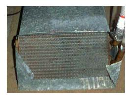
Here's a close-up of the heater core. If you don't know what a heater core is, it's basically a little radiator in your car's dashboard, and normally a pain in the butt to replace.
