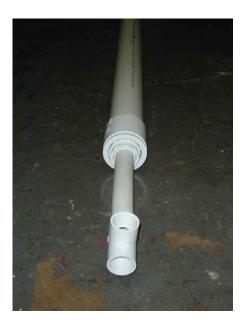
This is how the fog chiller should look when assembled. Once the chiller is assembled its time to fill it with ice.
