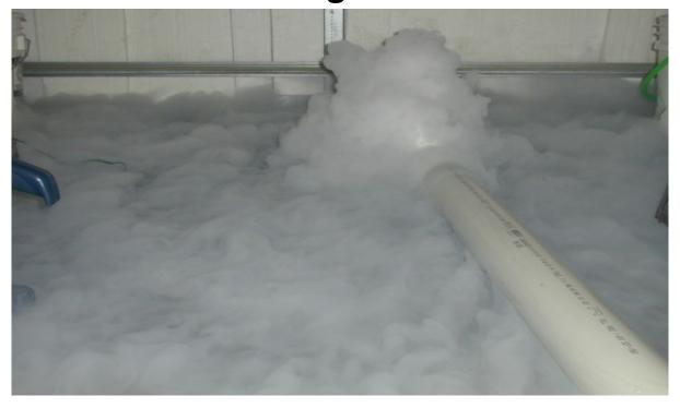
This is by far the simplest fog chiller I have built/designed. It's a snap to build as well. After assembled simply fill the 3" pipe with ice. Crank up the fogger and FOG!
