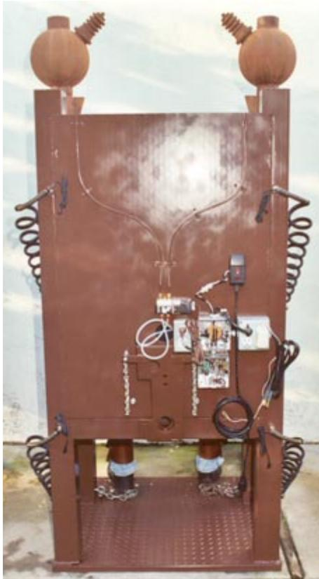
Here is a shot of the chair from the back. The Y-shaped tubes are 1/4" copper tubing which extend the exhaust ports of the solenoid valve to the top of the chair.
