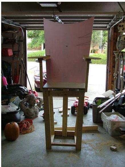
Once the frame was made, I cut out a piece of counter top I had as scrap for the seat and I used a piece of pink foam for the backing... I decided to put a 2x4 in the center of the back to help support the foam incase I leaned back too far.
