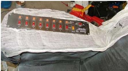
I cut out a hole in the arm of the chair (using a jig saw) to put in a light controller box so when I am in the chair I can turn on and off any other lights or electric devices I wanna use... (I.E. Strobes, black lights, colored lights, or my mic.)
