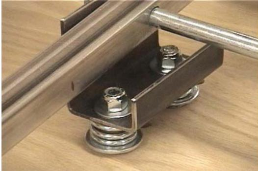
Remember to also place one of the rubber washers between the flat washer and the wood underneath the seat as well. Here is the spring assembly just before placing the leg assembly down to complete the attachment.
