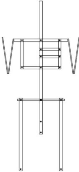
Here is a front elevation draft of our skeleton that will be made out of a combination of steel and aluminum to achieve a very durable, professional grade animatronic while keeping the weight down to reasonable levels.
