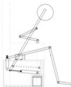
and make sure everything clears each other inside the seat as well as in the skeleton. In the first one, all is clear and working together, even allowing us enough space for the speaker under the raised floor section of the box. In the photo on the left we see that at the apex of it's cycle, both the skeleton and the air cylinder mechanisms are clearing by just enough to allow fluid motion. Success! Now it is only a matter of cutting some steel and aluminum!
