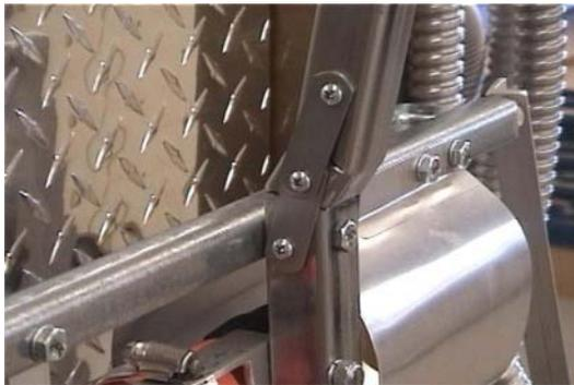
So to make our guy a little less rigid looking we will need to make a couple of cuts to the spine just above the shoulders. Cut out about 3/4" from the lower front cut as shown here and bend the neck forward to close the gap. Now remove about 1/2" from the cut just above that on the back side. You may have to play with this a little with your angle grinder to get it just right as I did, but the idea is to tilt the neck slight forward as well as moving it's center to the body forward slightly.
