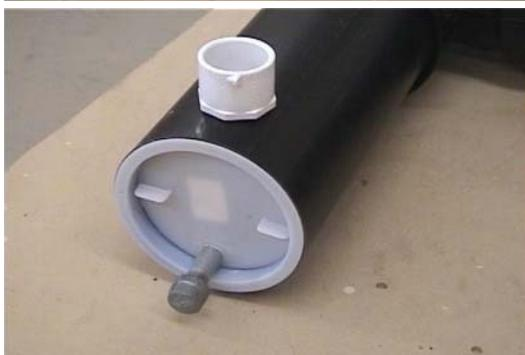
So we install this pipe with a thumb-tight cap on it so we can remove the decorative diamondplate cover on the right side of the pedestal revealing an opening we will cut into the wood side that will allow easy access to this drain pipe. Then it is only a matter of tilting the chair to the side and draining the excess unspent fluid away after use.
