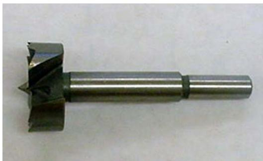
I used a 1 3/4" forstner bit (shown on your right) that drills a flat, blunt hole through wood as shown here to countersink the wood to accept the bump out of the T fitting. I will be using the same technique at the top of the front legs under the front of the arm rest right under the back of smokey's hand (shown on the left).
