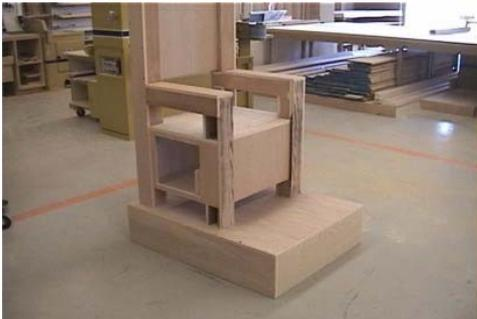
And there you have it. Position the chair to the back of the pedestal on center from side to side. You will be screwing (no glue) through the top of pedestal top into the legs of the chair to attach them, but remember that you will need to be able to remove the chair to complete the installation of the speaker as well as install the fog ducting up through the legs of the chair.
