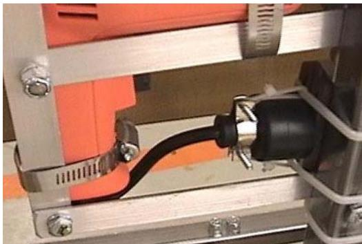
In keeping with the logic of making the drill in the chest of our doomed soul quickly replaceable, I shortened the power cord it came with to just 3" long and then mounted the female 3-outlet end of an extension cord solidly to the spine just above the bottom of the ribcage with heavy zip ties, then I zip tied the power plug of the drill to the outlet.
