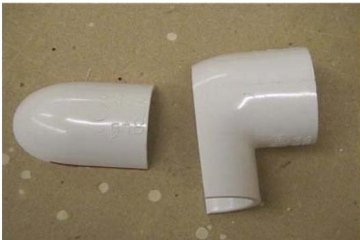
I decided on using a 2" PVC elbow that I cut the top off of. In the photo here you will see how I managed to do this without cutting my fingers off. I fitted a stick inside the opposite end to hold on to and then used a chop saw to nip the lid off. I then used two counter-sunk screws to attach solid to the chair.
