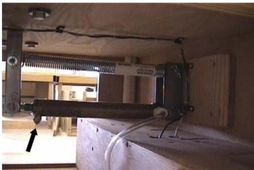
The cylinder I wound up using turned out to be a two way that I used an adjustable muffler on the unused port. You can see it in the photo (Left) where the black arrow is pointing.
