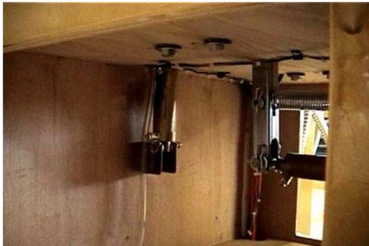
I used 5/16" steel rod for my connecting pins since this worked with my particular air ram. You can see it hooked up in the photo on the left.
