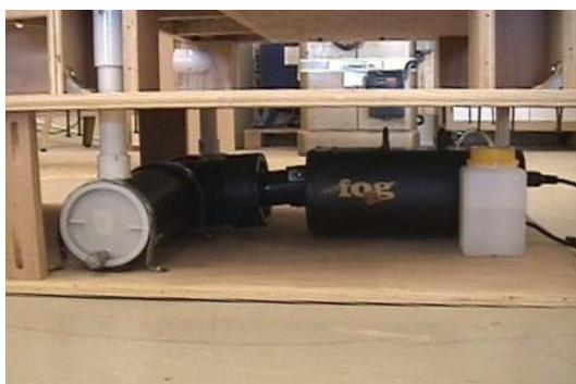
Now it is time to position our fogger assembly inside the pedestal so the fittings line up to the front chair legs. I use metal plumber's tape to clamp the expansion chamber in place and use a single L bracket screwed directly to the back of my fogger in a location that wouldn't harm the fogger.
