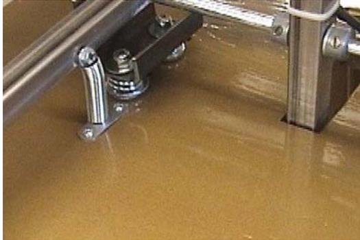
You will need to cut one of the looped ends off for the attachment system I have decided to use. Directly forward of the primary mounts on the seat, drill a 1/4" hole through the side of each leg and insert a 1/4" x 1 1/2" bolt using a flat washer through the top of the spring.
