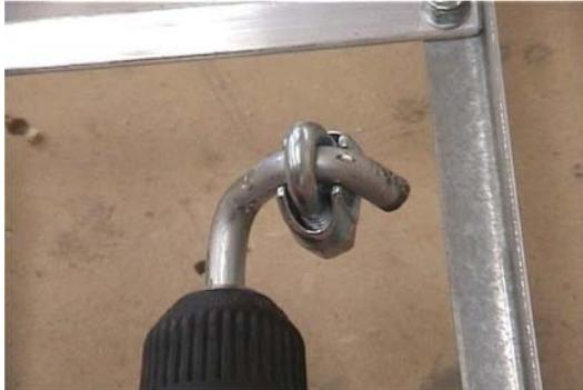
In the chuck you will notice our cam assembly. I call it an assembly because my original idea of simply bending over the end of a 3/8" steel rod wasn't heavy enough to really throw the chest around so I added a U bolt that is called a Clip that is normally used to attach cables. This added weight did the trick, so now it is only a matter of setting the trigger to the on position and turning the speed dial until the right speed is achieved for the most effective shake.
