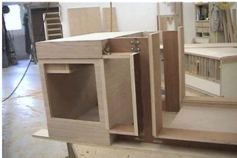
Another thing you see here is a 1 1/16" hole bored into the corners. This will allow us to not only get our fog ducting through the seat area, but provides ports for air lines and electrical wires. Drill all 4 corners at precisely centered to where the chair's hollow leg openings will be through both the floor and the top of the box as shown on the right.
