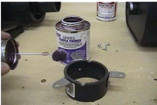
In the close up to our left we see the surface of the slip fitting that will be attached to the fogger has been sanded down on an angle to match the angle we will need to direct our fog downward and into the chamber. If you look close you will also see two notches needed to clear two tiny screw heads on the face of the fogger so our fit will be flush and perfectly sealed.
