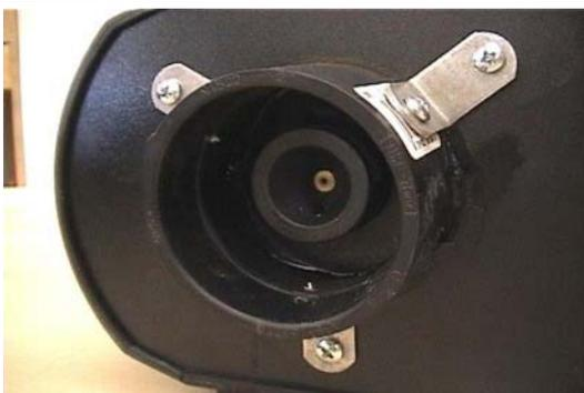
Next we attach the L brackets to the slip fitting with some screws so they will be flush or just above the bottom edge of the fitting, so we can pull the fitting down tight to the fogger face when the screws are installed.
