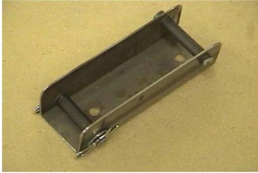
For the mount that will be centered on the back of the seat box below I made a clevis from a section of tube steel similar to the one shown here on the left. This particular double clevis was made for the connection of the torso air cylinder and it's return spring, but if you can imagine cutting this one in half and drilling two mounting holes in the bottom, you have what the clevis looked like for this leg assembly.
