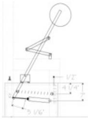
Above the air ram, 3 1/4" on the clevis and the lever I have shown a 12" spring that when installed will be slightly engaged, keeping the torso in an upright position when it is not activated and of course, bringing the torso back upright after activation. So at this point, it looks like we have succeeded with the first of the 5 animations our freaked out friend will hopefully wind up with. In this photo on the left you can see a close up of the mechanism.
