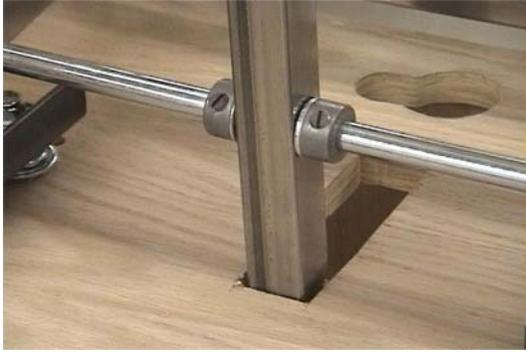
well to allow room for the nuts and rod end. Here is a picture of what it will look like once drilled and attached to the ram.
