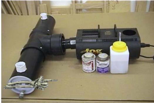
And there you have it! You will need to remove the fluid tank from your fogger so you will have a way to remove the tank from the pedestal to replace the spent fluid as shown here. This will be held in place next to the fogger with L brackets once we install our fog assembly.
