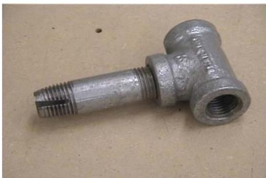
To thread the plastic of the stopper cap for our 1 1/2" length of 1/8" pipe we will need to make another tap as we did a moment ago. Here is the one I made, using a T fitting as a handle as mentioned previous.
