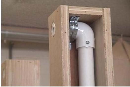
At the top of the back you can see how I am securing the pipe to the inside of the channel using conduit clamps that have been bent to the right form. On the front of this 90 degree elbow is a plug that I drill out one small hole in the middle of (this will all be covered with our "heat sink", so don't worry about the plug being visible). Once I tested the fog system, I wound up drilling the right hole a bit larger than the one in the left back, so start small with your test holes.
