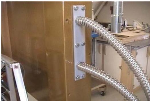
Here is a shot at the outside port I used to bring the power into the chair. This is a 1/4" thick steel plate that I have mounted flex conduit connectors to and then bolted to the chair with 1/4" lag bolts. The other end of these two power cords were fitted with turn-locking fittings you would find on high powered machinery such as a welder.
