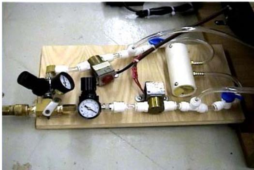
In the assembly shown here on a removable board (so I can get to all the components for maintenance), you will see I have installed dedicated air regulators.
