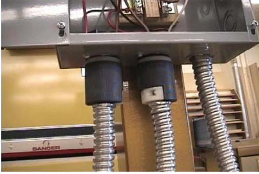
You can see the power outlets feeding them are mounted to the bottom of a small utility box that I decided to use as the executioner's power panel. The third leg on the right is the incoming power to the box and is mounted directly and hard wired in.
