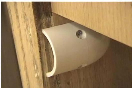
Inside at the back of the duct is the 1/4" hole drilled through the thin outer layer of wood and the PVC plug just behind it to allow a small amount of fog to exit. It worked beautifully and they were invisible to the eye once the paint was applied to the chair.
