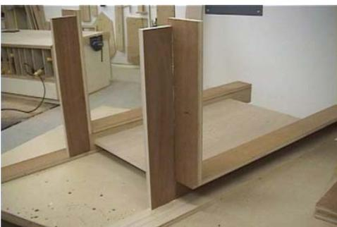
Notice that the top (H) is slipped UNDER the bottom edge of the front back stile A. Be sure to attach these two piece with screws and glue, as this is a critical stress point. I carefully predrilled two holes in the back of the lower piece as you can see here as I wanted this to be as secure as possible. If you don't predrill carefully you will split this narrow piece of plywood. For my connection of this piece,
