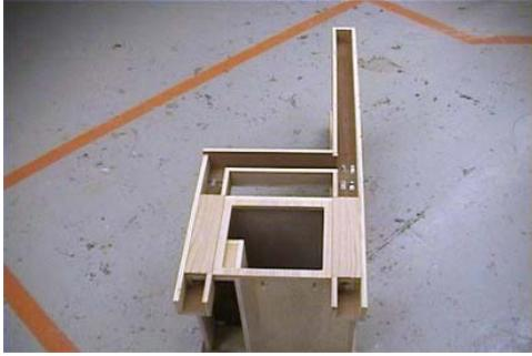
I used 1" x 1" brackets, carefully avoiding overlap of the holes in the seat. Here you can see the mending plates attaching the side of the armrest to the leg section. Now assemble your lower L shaped leg sections identically to the ones that went under the armrest using the 4 3/4" long pieces E and L. These can be glued and stapled to the rear back stiles B as shown in the photo below.
