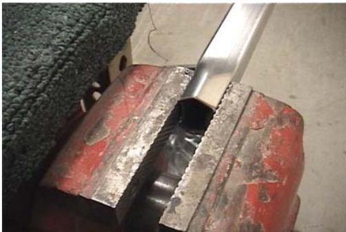
Next I place the top of the lower leg that will be the other half of the knee into a steel vise approximately 1" and slightly crush it just enough to slip inside of the upper knee slot. If you look closely you can see the lower pipe end just fits inside the slot to fully cover.
