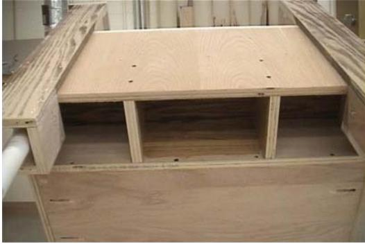
Next we need to set up a place for our powered computer speaker for the voice of our whimpering sissy. I tossed in some walls under the front of the seat where the floor was raised up to keep mine from migrating side to side and then I coated the cavity with contact cement.
