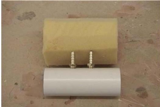
In the picture here you will see a short length of 2" PVC pipe that I will be using as a muffler for that bleed off. In one side I will drill and tap two 1/4" holes for air line slip fittings as shown already installed after tapping the threads with the tap we made in the previous section.
