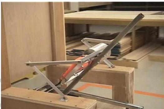
The mount to the chair is merely a short section of the same angle aluminum as the arms and is screwed down using two 3/4" x #8 pan head screws. This is 4" on center to the hinge pin from the front of the arm rest, centered. In this shot you can see how the skeleton looks now fully bolted down. And luckily the computer draft dimensions work out
