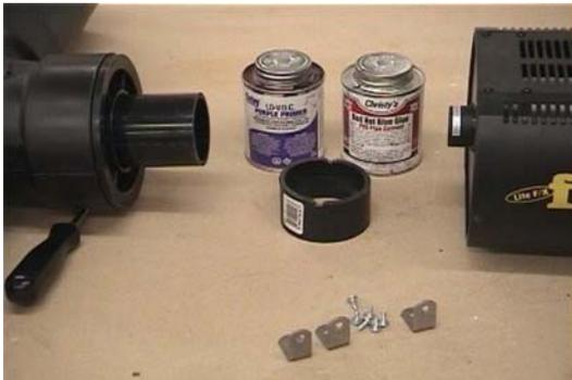
Here in the photo on the left, you will see the needed items to seal your fogger to the fog routing system; three 1" x 1" L brackets, some #8 x 3/8" sheet metal screws, a 2" ABS slip fitting, some PVC cement primer and a can of PVC cement.
