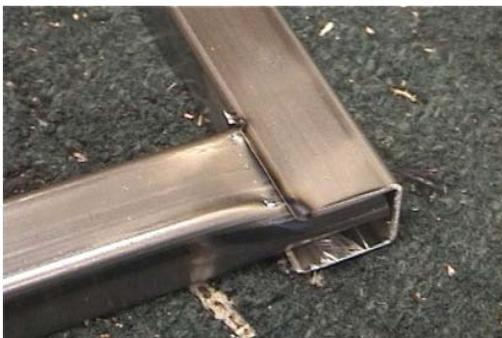
Since my dummy will be fitted with a foam rubber body, I don't want the knees tearing up the foam inside when he stomps his feet. The cover here should all but eliminate it from eating the body. Now I will round the bottom edges of the slotted end and attach the knee together using a hinge pin made with 3/8" steel rod that has been drilled out on each end for the hitch pins that will keep it together.
