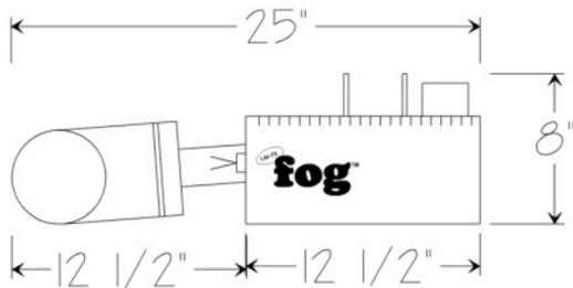
OKAY! We have moved on to one of the more interesting sections of our project, the [Vortex Fog Delivery System™](#) which I developed at the turn of the century to move fog without using fans so the resulting fog is much thicker than it would be otherwise. This early version of the system shown here is fully sealed which I installed in the pedestal of the prop, making this a fully on-board event.
