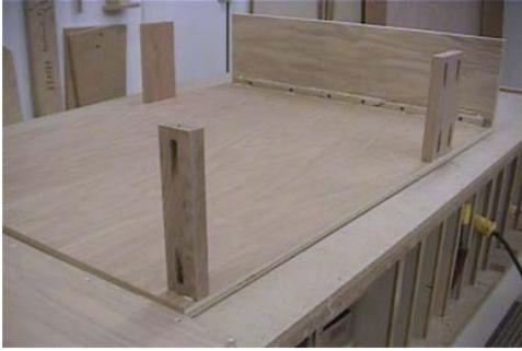
The pedestal is a fairly straight forward box with a hinged rear door that will be frenched in below the top and above the 3/4" floor. I used a 3/4" X 3/4" glue block to attach the front to the floor as you can see in the picture on our left. As mentioned earlier in the how-to, I am using some solid oak braces that will be attached to the top and the floor that will allow me to remove the sides of the pedestal should
