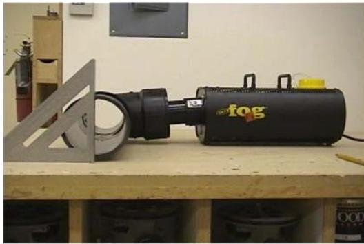
In the photo to your left I have set up a carpenter's square to mark the exact top of my 5" pipes so I can drill holes and thread the pipe wall for 1" PVC fittings I will use to attach the ducting that will run through the chair.
