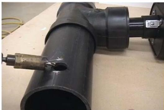
I have measured to the center of where the pipes will be coming up through the top of the pedestal and through the front legs of the chair and used a hole saw to drill my pilot holes in preparation. Next I will need to make a thread tap for this size pipe fitting.
