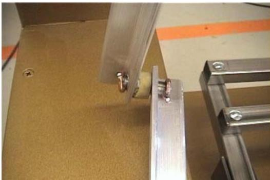
Between each hinge point of the arms I placed a short section of 3/8" rubber air line as shown here.
