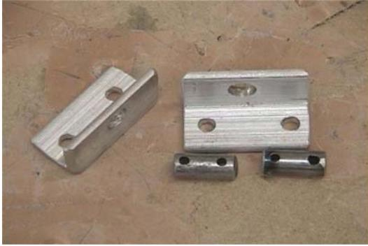
You will need to make six 1/4" hinge pins out of solid steel rod for the arms of our whiner.
