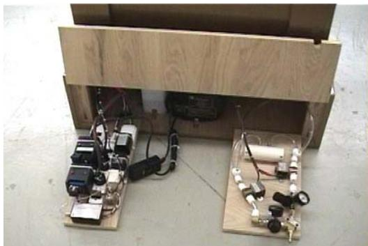
Here you can see what the rear of the chair and pedestal look like with the panel assemblies slid back and the hinged door up. At the top of the door notice the notch that will allow a 3/8" air line to pass through while the door is closed. For more info on setting up the use of sound and timers, go to [Motion Trigger](#).
