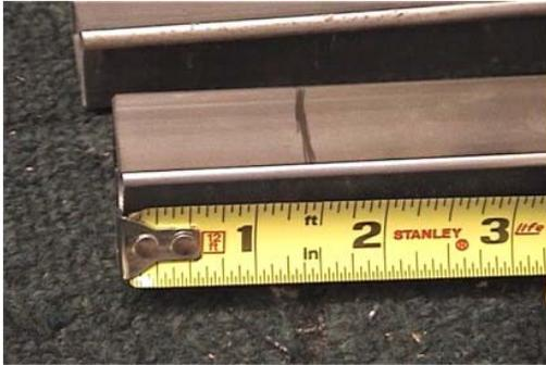
Using 1" square 1/8" wall steel tubing (don't ask me why the steel industry calls square shaped steel "tubing", as I still can't figure it out myself)
