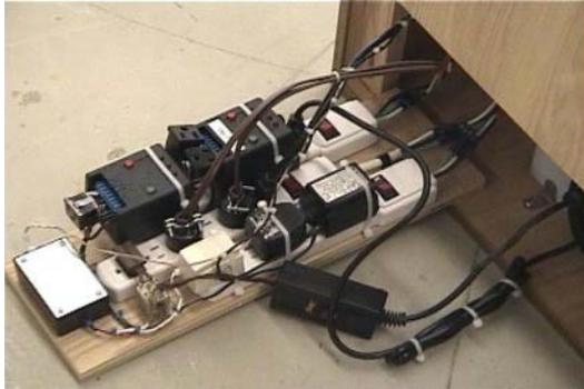
conduit, so this is the logical placement. These are held in place with screws that each strip locks into in the back.
