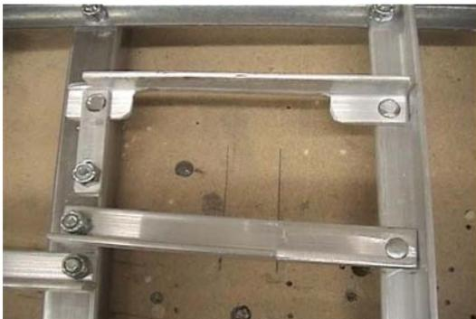
You can see this is where you will be attaching your angle aluminum which is a total size of 9" high and of course 12" wide. On the right side of the cage you will be attaching two 5 7/8" pieces as a mounting platform for your variable speed drill to rest on.
