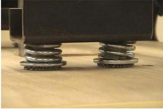
Called 5 /16" Tank Bolt Washers and made for your toilet tank connection, you can find these in, you guessed it, the plumbing section of your local hardware store! These will be placed underneath the bottom washer below the spring to keep the steel washer from coming into contact with the wood which would eventually wear through if left in contact. Hopefully with this layer of belted rubber this will never be a wear point on the chair.
