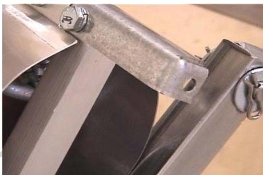
Next we drill a 1/4" hole into the 90 degree tab at both ends of the shoulders.
