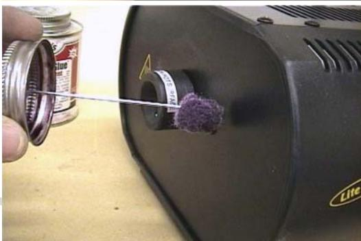
Then clean the mating edge of the fitting with your primer and also the front of the fogger where they will meet. This will emulsify the surface of the plastic face as well as the fitting so when we apply the cement, we will be bonding to the plastic on a deeper level than just surface only, making sure it is a secure bond. Pre fit the the fitting centered to the nozzle prior to gluing so you are certain of your placement. Then of course glue the two surfaces and attach with screws.
