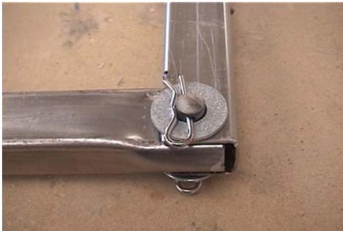
The limited movement of this joint turned out to work perfectly for my needs on this prop, so I simply created the same type of joint at the bottom of the lower leg to function the same way for the ankles.
