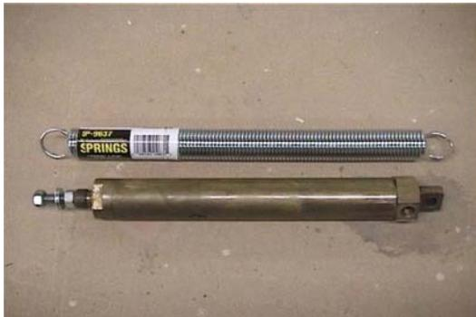
As mentioned earlier, the air cylinder I chose for the torso is a 10" air cylinder that is overall about the same length as this 12" spring, making them perfectly compatible for actuation and return. The spring came from Home Depot and the air cylinder is a Bimba brand as mentioned purchased from surplus. Here is a close up look at both.
