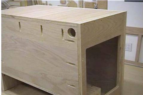
Here is what your box will look like once you put the sides on. I cut out my openings before assembly, as you can see there is in fact a small amount of the raised floor that is exposed to the opening, keeping us from being able to make this cut out after the box's assembly.
