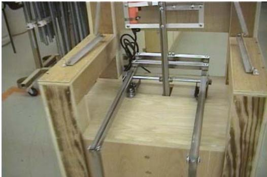
The upper arms will be 10 1/2" long, made out of 3/4" x 3/4" angle aluminum as will the lower arms cut to 11".
