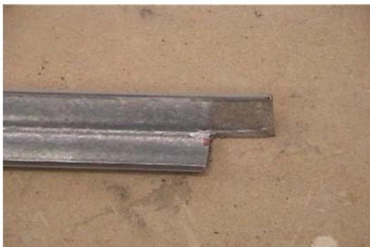
For the rib cage assembly we will be using a combination of 3/4" x 3/4" x 1/8" angle iron and 3/4" x 3/4" x 1/8" aluminum angle. To start we will cut out 18" of the iron and notch one of the surfaces back 3/4" as show in the left photo.
