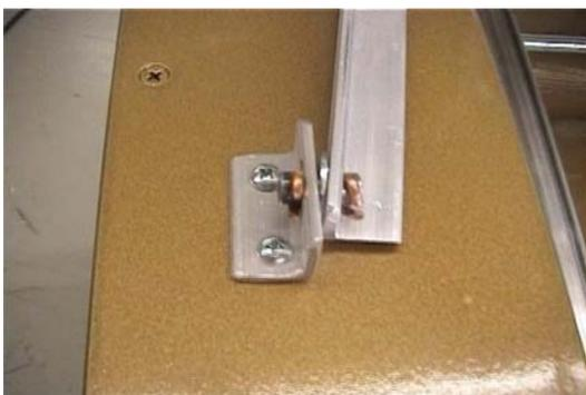
At the ends of the hinge pins I drill a small hole and insert a short section of heavy wire that I simply bend over.
