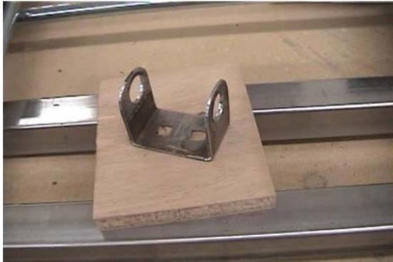
Now that our leg assembly is built, we will need to add a clevis mount to the bottom of the rear brace as shown in the photo above. To achieve this I cut the top off of a 1" X 2" piece of tube steel and then chop off 1" of the larger bottom section. I rounded the top edges and then drilled a 1/2" hole through both pieces now sticking up to hold the 1 1/2" piece of 1/2" solid steel rod I will be attaching my air cylinder to.
