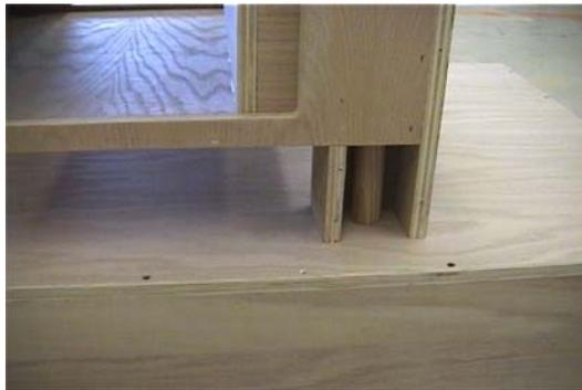
So we will need to determine where our fog ducting will go through the top of the pedestal in order to be perfectly centered to the front chair leg channels. To do this I use a 1 1/4" diameter dowel that I dropped down through the hole in the seat box floor to make my mark. While I am at it, I drill the holes lining up with the back legs of the chair as well, since I will need to use those openings for my air lines and electrical cords as mentioned earlier.
