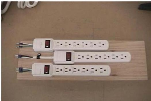
For the electrical needs of the chair I have decided on a bank of three power strips tucked in tight side by side that will fit between the fog juice bottle inside the pedestal and the wall. This will be removable just like the air assembly on the opposite side of the fogger. I will be running the electricity into the right chair back post through flexible
