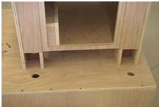
Once I slide the chair aside I can drill these holes using a 1 5/8" diameter hole saw.
