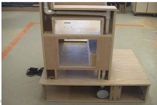
This is the other side of the chair where you can see the fittings already in place going to the wrist and then back to the back posts. All of these fittings can be screwed together using 1/2" x #8 sheet metal screws instead of glue in case you need to adjust them for any reason.
