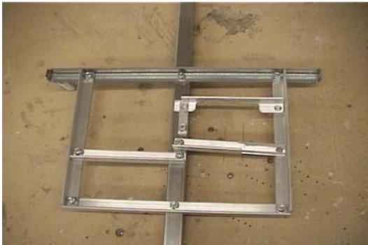
Do this to both ends and then attach the iron to the front of the spine 11 3/8" from the top. This is the dimension to the top of the angle iron. Use a 1/4" bolt with a lock nut.
