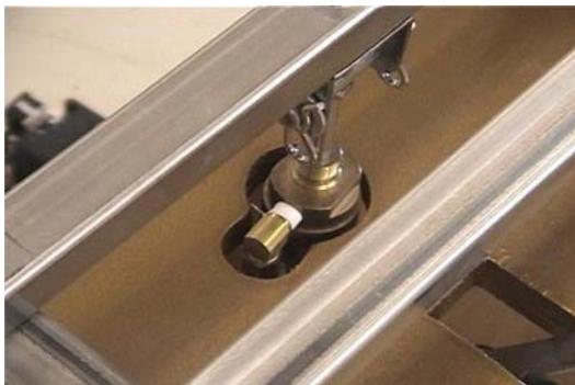
For the rear connection of the leg assembly to the air cylinder you will connect the cylinder to the connecting pin and drill for the safety wire through the nut and the rod as shown earlier in our how to. When I went to install this one, I found that I needed to send the air into the cylinder at the top, so I had to drill another hole in the seat to allow for room for the air line to pass through next to the 1 1/16" hole needed for the top of the cylinder .
