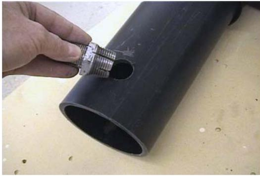
Once it did, I turn it down with a crescent wrench until I have buried the tap as deep into the pipe as I could to make sure the threads are fully cut and clean inside the hole. And here you see the 1" PVC threaded fitting (male end) to a slip fitting opposite threaded securely into the holes.
