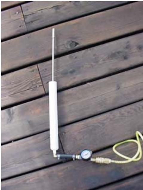
For testing I put a small regulator in-line and started working up the pressure until I found a good action that was not too rough on the piston. Anything below 30 PSI was barely enough to move the piston. I ended up at about 55 PSI and it has a really good action.
