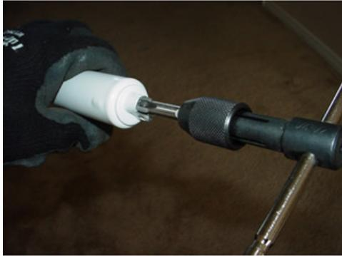
Next step was to drill out the existing hole and tap it for a 1/8 inch pipe thread. I kind of guessed at the pipe size while I was at the store and it turns out that 1/8 inch pipe thread is perfect for the hole.
