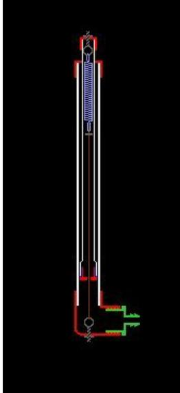
If you're looking for a fairly inexpensive way to build long throw pistons (12 inches or more), then the PVC pneumatic piston is the way to go. They're powerful enough to lift about 10-15 lbs at 40 psi and only take about 1/2 hour to make if you have the proper parts & tools on hand.
