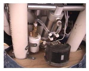
Here is yet another way to use your compact muffler. These photos, which was first used in the 2003 project, the Lynching, shows a second fitting on the top side of the muffler that can be used to silence the exhaust from the secondary air inlet on a 2 way air ram. You must route these two lines into the muffler separately, as if you link them together, you will in essence be attempting to force air into both the PUSH inlet and the PULL inlet of the same air ram.
