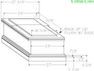
This is the coffin shape I decided on after much thought. The box of the casket itself is assembled by attaching 3/4" x 3/4" trim on both ends of the front and back pieces of plywood. Once the trim has been woodpatched and belt sanded flush to the plywood, we will glue and nail the front and back pieces to the side pieces in a butt joint. After gluing and nailing the box together, woodpatch these joints and well and belt sand smooth.
