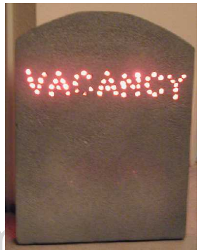
Red Chasing lights were used for a twinkling effect
