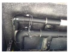
To the left is the picture of my homemade grommets. I just cut some plastic strips out of some old containers and poked holes in them, then slid 12 gauge wire through them into the foam then around the PVC under the roof to hold it together
