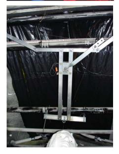
In the this picture, you can see the FCG rig in place. I use some scrap sections of chains placed along the top brace sections of PVC on the crypt to hold the FCG up. I wrapped the 4 pieces of chain around the PVC and used zip-ties to hold them together, then I used caribiners to connect the chains to the eye bolts on the FCG rig.
