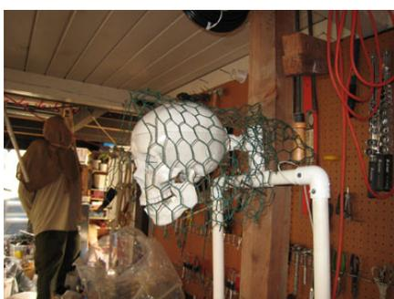
To make the bracket for the head, I took a T, cut it in half, and then flattened it out by blasting it with the heat gun and putting weights on it until it cools.
