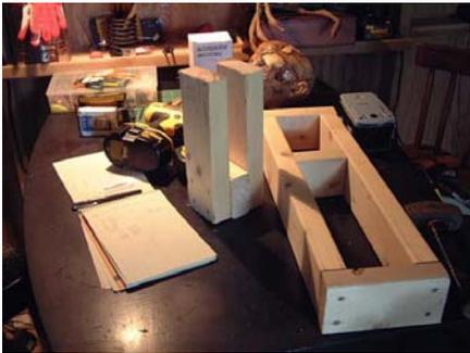
Cut two additional blocks at 3 ¼" and wedge them into the box (fig. 3), these will act as the upright and servo tray supports. Cut two 10 ½" inch pieces and a 5" piece of the 2x4", screw them to the front 3 ¼" block as shown to serve as the upright support.
