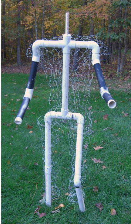
The frame is 1.5 inch PVC pipe and fittings with chicken wire to provide some "body". The frame is slipped over iron re-bar driven into the ground. The 1/2" PVC neck is inserted into a reducer fitting placed in the 4-way fitting. Here's a great [calculator](#) that can help with proportions.
