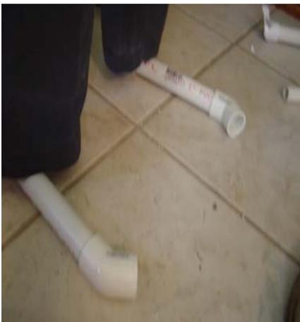
Next I add a length of PVC onto the end of the leg for a "foot".
