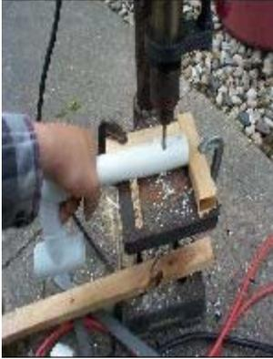
one end to lock the flat stock in place, and one on the other end to act as the pivot point for the joint. If the armature is to hold something or seems to be slipping I add a 1 1/2" piece of wood dowel with a hole drilled through it into the PVC at the pivot point to make the joint lock in place better.
