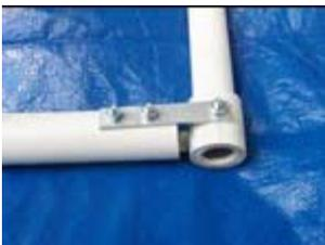
The next step is to add side-to-side movement to the arm. This is accomplished by inserting a 1" by 6" piece of PVC three inches into the upper arm that you just made. Then drilling a hole through both by drilling about 1 1/2" from the bottom of the 1 1/4". After drilling the hole its time to make another slot. But I bet you already know that. Once the slot is made reassemble the slot joint and you are on to the Elbow.
