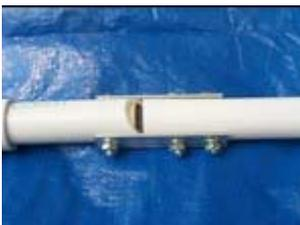
To make the elbow you need two more 4-inch pieces of flat stock. Place them at the end of our arm assembly and mark for drilling. Once drilled fasten and tighten with a 1 1/2" bolt. For this joint you want the two pieces of PVC to butt up as you are marking them for drilling. If there were
