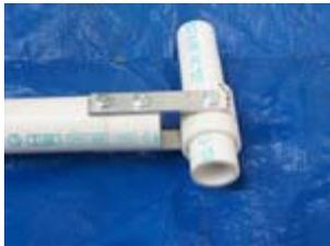
I slip a 1  $\frac{1}{4}$ " by 4" piece of PVC over the end of the leg assembly and attach the joint to it. Then the other end of the joint is attached to a 1" tee connector. The final step for the leg is to add the foot. It is just a 1" by 4" piece fitted to the end of the tee. Once both legs are complete take the 1  $\frac{1}{4}$ " 4 way connector, insert a 1  $\frac{1}{4}$ " by 2" piece into each apposing side and insert each leg assembly. After you do so check the
