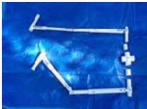
After that is completed it is on to the next and last slot joint for the leg. Insert a 1" by 8" piece 4-inches into the leg assembly and drill a hole about two inches from the bottom. Next make the slot. This will allow the leg to bend from side-to-side. Once done its time to make the knee joint. That is done the same as the elbow by butting up the leg assemble to a 1" by 14" piece of PVC and making the
