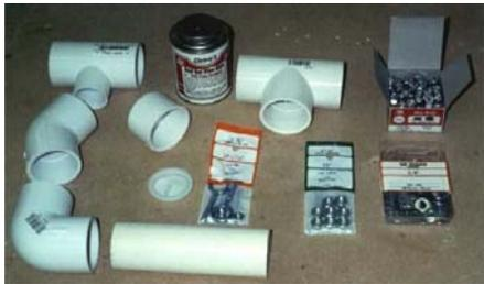
In the photo here you can get a good look at much of the items needed for the skeleton of your dummy. It is fair to note that the need for the PVC adhesive is purely to adhere the caps that cover the openings in each side of the hips assembly. This is not needed and can save you a few dollars off the cost of constructing this guy.
