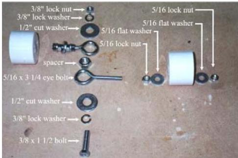
Before our dummy can begin to take shape, we will need to assemble all 12 of his joints. This will entail preparing the pipe cap fittings with the necessary 5/16" hole in the center of each. Also you need to assemble the joints and attach them to each cap.
