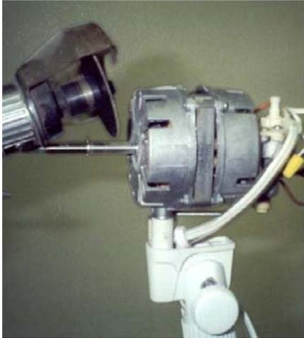
Now we will cut off the nipple that sticks out that the fan and cage attach to. You can use a hacksaw for this or a pneumatic cut-off tool. Once you get to the fan blade shaft itself you will have to hold the shaft with a pair of vise grips to cut it off with a hacksaw or a die grinder cut-off tool as shown here.
