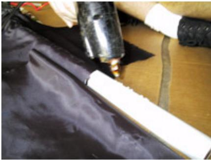
We have 3 foot long by 1 foot wide strips of black fabric that we hot glued onto the pipe.
