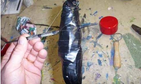
Pierce through the body with a sharp object. I used a dental pick, but any object that can poke through the tape and paper will do. I suppose a standard ice pick would also work great.
