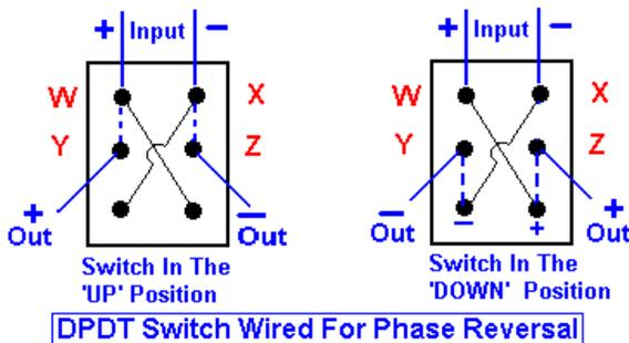
Now let's see what happens when the switch is in the 'down' position (right diagram). The + input goes from the 'W' terminal, down to the lower right and then up to the 'Z' terminal. The negative input goes from the 'X' terminal and out through
