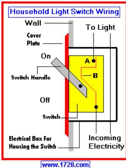
This type of switch (having a lever which "flips" it on and off) is called a toggle switch.
