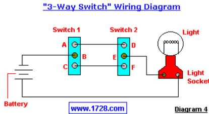
So, how does this work? Let's say that Switch 1 is at the bottom of a stairway and Switch 2 is at the top. Suppose Switch 1 is in a 'down' position (B & C connected) and Switch 2 is in an 'up' position (D & E connected). The light bulb is off. Now someone comes to the bottom of the stairs and flips Switch 1 'up'.
