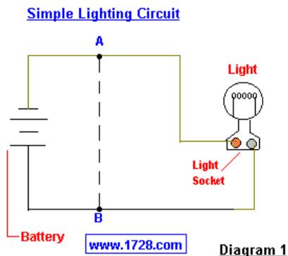
Diagram number 1 illustrates an extremely simple circuit. (For the moment, ignore the dotted line and the points A and B). The battery is represented by 4 lines (the longer line being positive and the shorter one negative). Starting from the negative end of the battery, electrons "circle" through one wire, pass through the light bulb, pass through the other wire and then return to the battery thereby completing the circuit. See? Quite simple.
