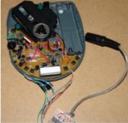
**Drill small holes in the case of the CD player to run the wires through.**
