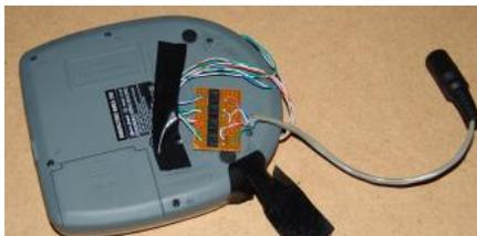
From there, solder those wires to the transistor side of an optoisolator. The important thing to remember here is that polarity matters. You need to determine which wire is positive and which is negative so that you can hook it to the transistor properly. If you do it backwards, it won't work, although I don't think it will hurt anything. Use a voltmeter for making this determination.
