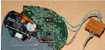
Take the CD player apart and find the solder joints of the various buttons (play, stop, etc.). Solder a wire to both sides of the button. By doing so, if you touch the other ends of the two wires together, it's as if you pushed the button.
