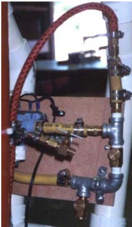
Now we need to mount the air system to the back of the chest cavity. I used a small piece of 1/4" board to mount all this on and screwed it to the frame. Since you have already assembled your air trigger, mount this on the top left of your assembly plate as shown in this picture.
