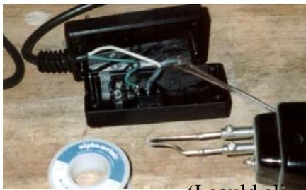
Since I determined that it is indeed a passive circuit, I simply solder a remote wire to each lead of the switch legs
