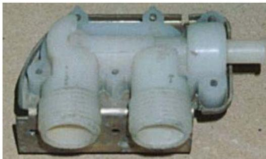
Of course you will need a water valve from a washing machine and not just any valve will hold the air back and reseal itself under the rather high pressure I would need for an air cannon. I wound up testing many, many different valves to see which work and which don't. There are two that I have had success with at high pressure such as what my [Aerial Executioner](#) operates at, some 85 lbs.
