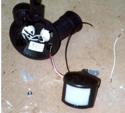
First thing is to disconnect the detector from the rest of the assembly as shown here. There is an extra length of wire that is used in the attachment to the light sockets that you will want to save for the next step. On close inspection of the photo you can just make out two wire couplers on the lower left. One is for coupling two small electrical wires and the other is one size larger that accepts three wires.
