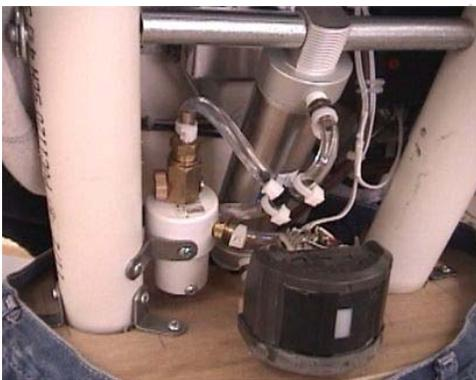
Here is yet another way to use your compact muffler. These photos, which was first used in the 2003 project, the [Lynching](#), shows a second fitting on the top side of the muffler that can be used to silence the exhaust from the secondary air inlet on a 2 way air ram.
