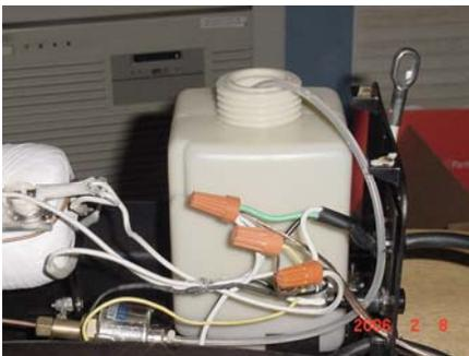
Basically I just identified the wires that fed each side of the switch on the remote, traced them back into the unit, and added my own leads to the wire-nut bound connections. I drilled a small hole out the back of the unit to feed my new wire, and ran that wire to the K1 blocks on the RC-8 board. Here's a close-up of the innards of the fog machine with my new leads attached;
