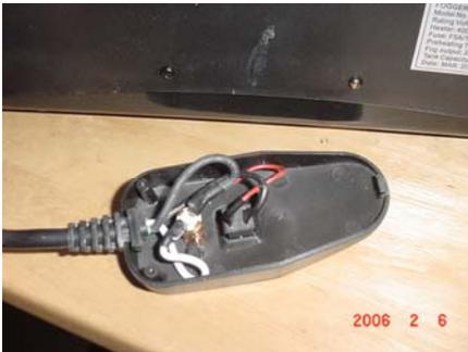
So, I opened up the remote and the unit to determine how the switch worked. I have several similar units, and the wire colors inside the units are different on each, so if you try this yourself, don't go simply by the wire colors on my unit.
