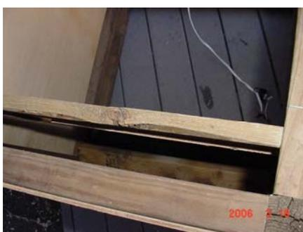
Next we built a drop-in wall behind the front wall that will channel the air up the inside front of the well. I left a gap in the middle of the inner wall (partly on purpose to route fog into the channel as well; partly because I used two scraps of wood I had leftover for the channel and they didn't cover the entire width.)
