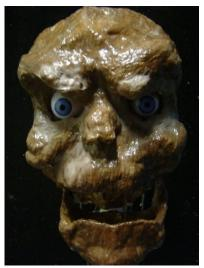
This is my latest project called spare parts because its made of stuff that I had laying around. Its also a training project to learn how to control servos using a basic stamp. It has 6 servos so far. The eyes have 2 for up & down and Left & right movement. There is one servo for the mouth and two for left/right & front/back tilt. Then the last turns the head from left to right.
