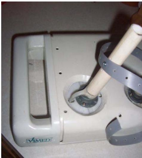
Step 4 - place the PVC pipe over the metal pole on the massager, with the securing screw facing out to the end of the massager and the short length of tape on the left of the PVC.
