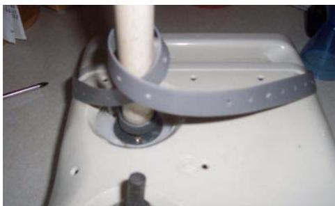
Step 7 - Switch on the massager to make sure that the PVC armatures move freely and don't lock up - if they do you will need to adjust the securing screws further down the tape either side of the PVC to give more slack.
