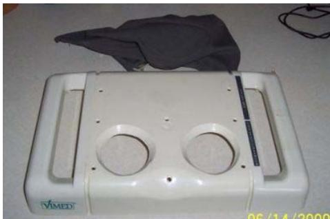
2. remove the top of the shiatsu by removing the screws underneath, then remove the fabric by taking out the screws or clips holding the fabric (this is my preferred method and will help with step 2).
