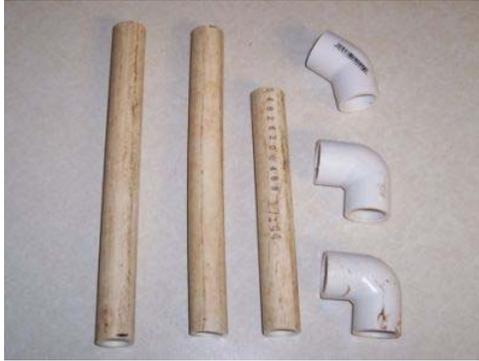
For the final steps of the basic grave grabber you will need the Head and hand, two lengths of PVC pipe each 8" long and one 6" long and the fittings
