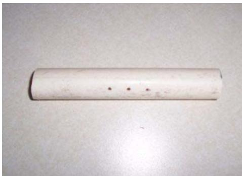
Step 2 - Next, on the two lengths of PVC pipe I drilled 3 holes 1/2" apart. The lengths of PVC used were 5" long and the centre hole drilled half way on the PVC
