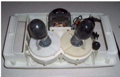
The two rubber nodules need to be removed from the rotating poles. These can sometimes just be pulled off by hand, or pried off with a screwdriver. Be careful when prying off as they have a tendency to spring off with a high velocity.
