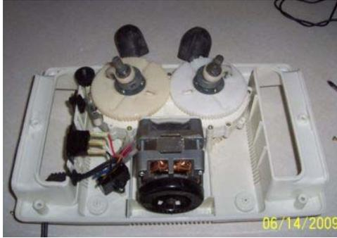
However, as in the case of this particular model the rubber and poles are one piece and will need to be cut away using a sharp knife. You can see where the cut mark is in the second picture the nodules removed
