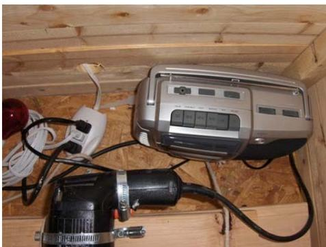
I'm not sure if you can tell here how the mechanics works. The drill spins the arm I have attached and rises up and down which makes the lid of the box open and close.
