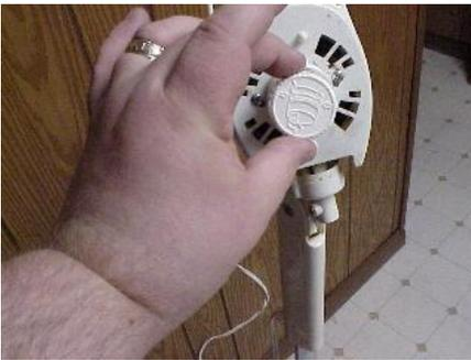
At this time test the fan and make sure that there is nothing rubbing together. Remember rubbing together = friction = heat = possible fire! In this instance, I used the cap from the bottle of "NyQuil".
