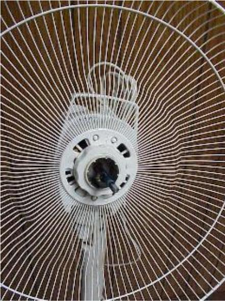
5.) The cage cap is unscrewed and removed.
