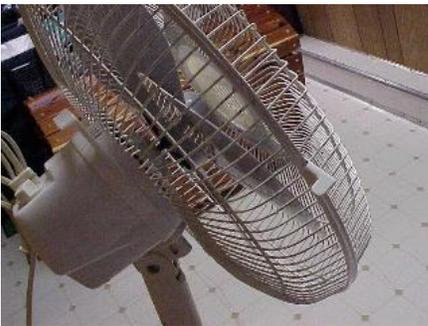
2.) The front half of the cage for the fan is unclamped and removed.
