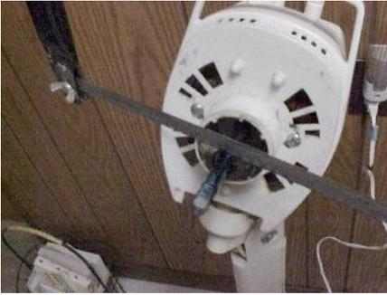
7.) The axle that the fan blade uses is then cut off with a hacksaw.
