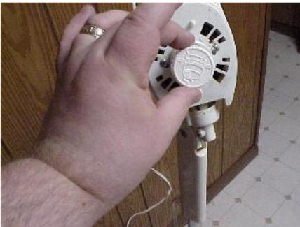
At this time test the fan and make sure that there is nothing rubbing together. Remember rubbing together = friction = heat = possible fire! In this instance, I used the cap from the bottle of "NyQuil".
