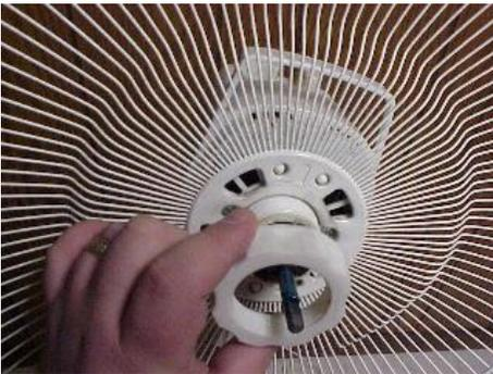
6.) The back half of the cage for the fan is now removed.
