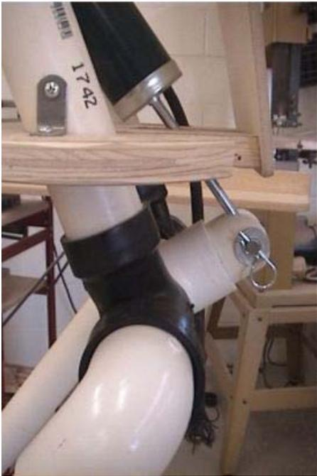
You will need a piece of 1/4" plywood or fiberboard as you see used here for the back to not only keep our skeleton together but to give us something to attach a large amount of electronics to. Notice how the waist is angled to meet the back. You can use #8 X 3/4" screws to attach this to the PVC and waist. The photo on the left shows the legs elevated with the lever fully deployed to show the end will just touch the back of the pants of our su
