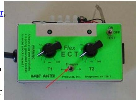
for, say, 20 seconds. If you run two wires from your solenoid, or Interface, to the side attachments on this ECT it will detect the circuit closure and send 110V power out of the power outlet on the right side of your picture and to your Jezebel.
