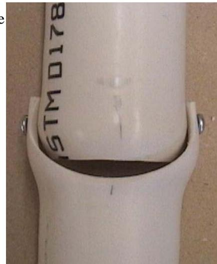
If you look closed not only is the end of the upper piece rounded at the end, but the inside of the lower part is belled out and the inside edges
