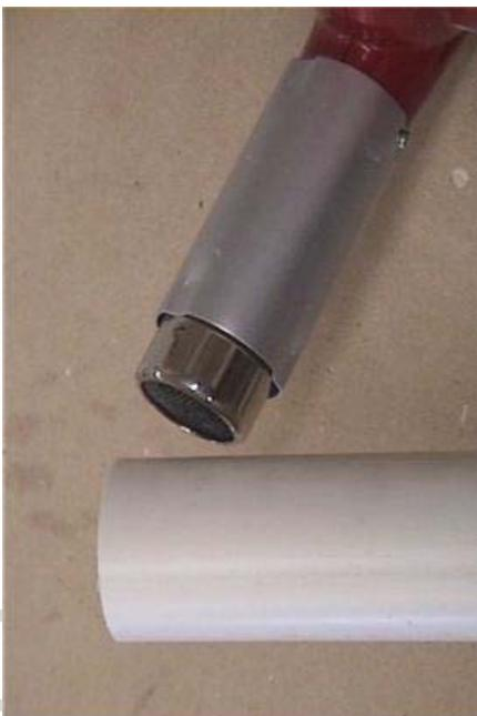
To round the end of the upper section I used a wine glass, as it had a rounded bottom inside and I need to use that as a mold for the plastic. The heat gun brought the PVC up to a soft, pliable point in just a couple of minutes and I simply pressed the end to the bottom of the glass and held it there until the plastic cooled.
