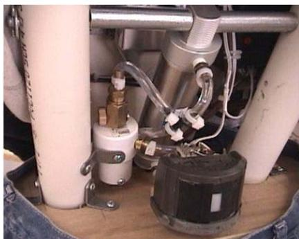
It turned out the air cylinder we used was double acting, which means it will push or pull the plunger.
