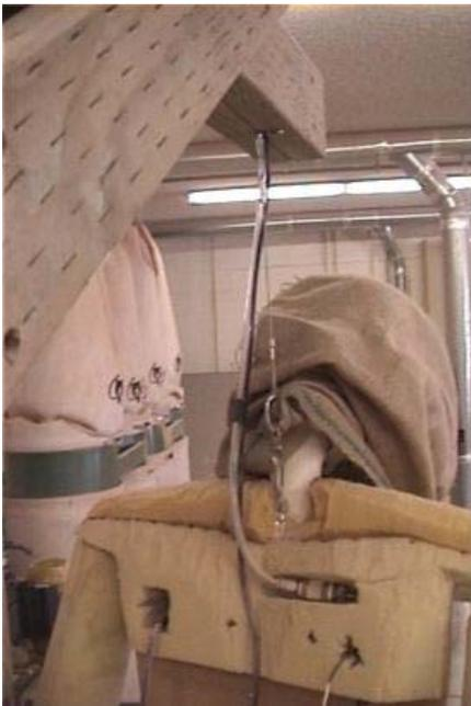
When you hang your dummy up make sure you zip tie your air, electric and steel cord together to prepare for the rope wrapping. And be sure to use a heavy gauge eye bolt in the gallows for the steel cord, as this guy jerks pretty hard against the connections.
