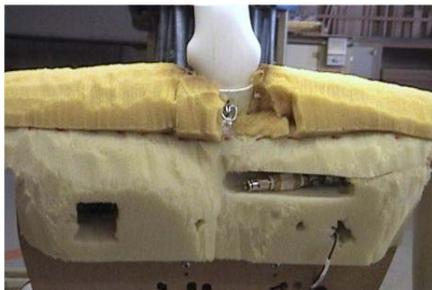
Here is another look at the back of our dummy where you will see that the PVC pipe neck has been heated up with a heat gun and bent forward to imitate the slouched forward head of a hanging man. This is about a 20 degree angle shown here.
