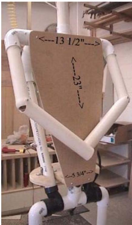
Three slots will need to be cut out as you can see for the wood to slip over the PVC pipe and the plunger from the air ram.
