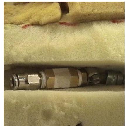
It is fitted on the end with a quick connect for 3/16" O.D. vinyl hose, also making it easy to detach if we want to take our boy down for any reason. In the left pic is the square cut-out in the foam where we have fitted a hard-mounted female 110 V electrical cord outlet we recycled from the back of an old tape deck, which is soldered to the shortened end of the power strip on the
