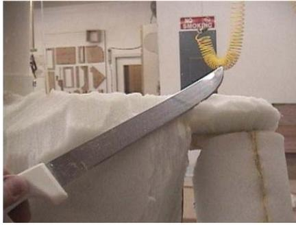
Using a serrated kitchen knife I sculpted the foam to roughly the shape each part of the "body" should look and kept adding additional foam as needed to get it to really bulk out.
