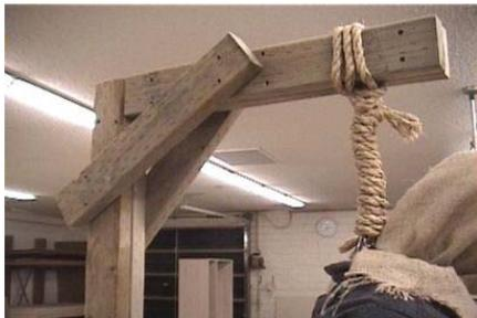
Now you can lay on the mating pieces of both A and C and screw together using 2" drywall screws. Don't worry that these pieces are not glued and screwed at the joint like our first half was, since the strength of that one joint along with the support of the angle pieces (B) will be more than enough to support your dangling dead dude.
