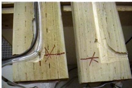
Here's how you will want to mark where you will run your 3/8" Cove bit in your router; in pieces A, mark a turnout where the lines will drop out of the wood at about 5" before the very end where the guy will be hanging from. Then mark all the way down the center and out the end of each. Above is a shot of the bottom of pieces C.
