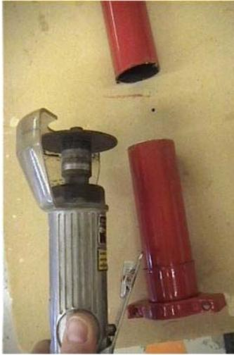
I learned that this foot pump will not work as an air ram, or at least won't continue to work at the pressure level I had to use to trigger the event here which was 28 pounds. For some reason the air began right away to leak past the seal and the cylinder was rendered useless in only a few cycles.
