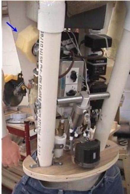
This is a panorama of the completed guts of our spastic friend after replacing 2 timers in search of one that would really make the actions of the jerking believable, adding yet another event control timer to control just the voice due to the ghost signaling we were getting, replacing the pressure regulator, replacing both the powered speakers for the large one at the top of the pictures and the replacement of 2 air rams.
