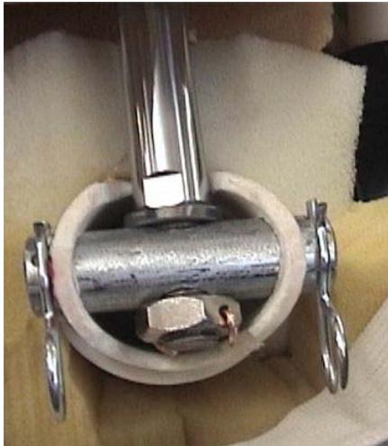
The massive plunger on this air cylinder that was mentioned at the start of this how-to, is 3/8" in diameter! So out of the lever comes the old steel rod, the PVC lever is drilled out with huge 5/8" holes and a section of 1/2" electrical conduit is drilled and fitted for the ram's plunger and the hitch pins.
