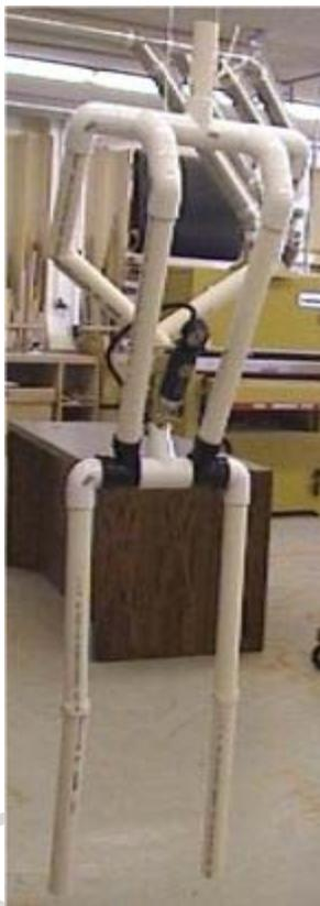
Now it is a simple matter of attaching the two 90 degree "hip" elbows to the 5" sections of pipe that go into the center 1 1/2" T fitting.
