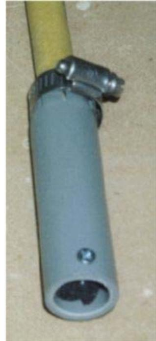
NEW! The new "compact" muffler shown here uses 1" PVC pipe just 2 1/2" long with one end capped and threaded for the valve you see installed.
