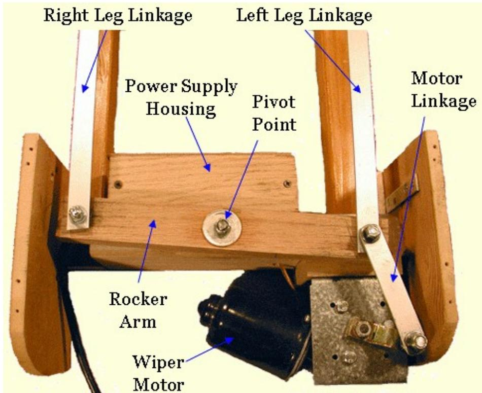
The leg linkages connect to the rocker arm using 1/4" bolts, t-nuts, washers and nylon insert lock nuts. The bolt and t-nut is shown below.
