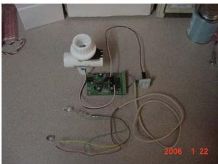
To the PROP1, I've wired a PIR (passive infrared) motion detector, a pair of LEDs to light the eyes, the servo, and a sound board (Radio Shack digital voice kit).
