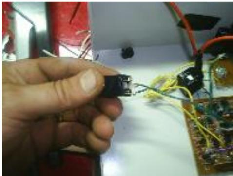
Here is the motion sensor. I drilled a hole in the case for it. As people walk by it should start the hangman kicking.
