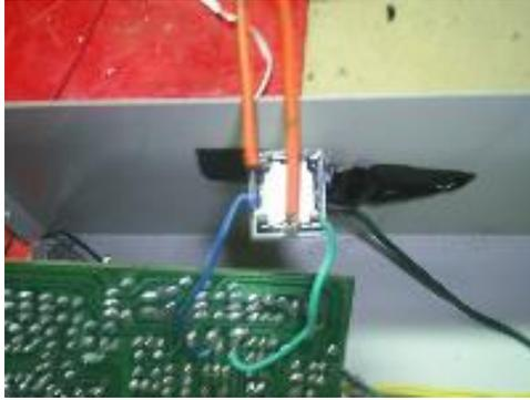
Wires were soldered to the relay to power the wiper motor that will run the hangman. The wiper motor is powered by a 15V 1 amp power supply. One wire from the power supply goes to the wiper motor, the other goes to the relay. The other wire on the relay will go to the other wire on the wiper motor.
