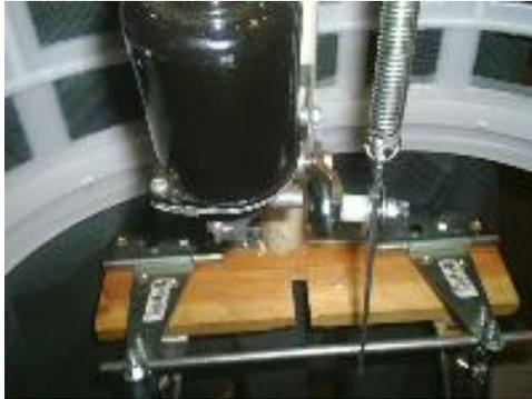
Here is a close up view of the wiper motor and kicking rig. Notice that I added a counter weight spring to the motor. It took a few times to adjust the spring for the right tension.
