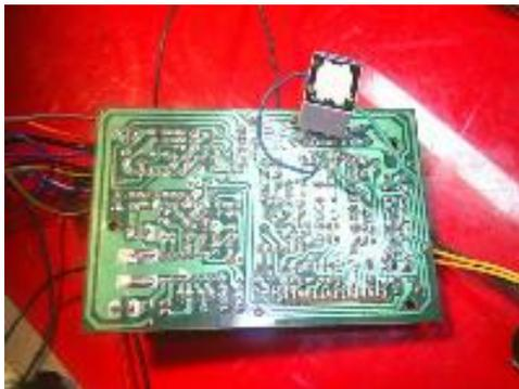
On one side of the board are the wires that work the Santa motors and the speaker. I remove them here to show the blue and green wires. I connected them to a 9 volt relay.
