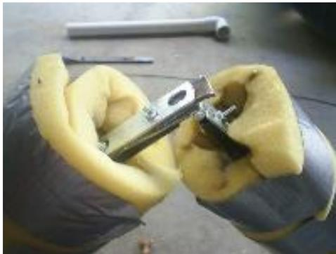
Close up of the knees. they are just hinges. I placed a piece of metal over the top stop the leg from bending one way.
