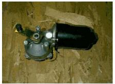
The heart of the Hanging Man is the Saturn windshield wiper motor. This is one of the most versatile motors I have come across. They are available at a variety of surplus houses on the net for under \$20.00. It operates as high as 106 RPM, and can be slowed down by either the internal switching, or by reducing the input voltage to 6V DC.
