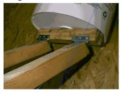
Measuring the bottom of the pail, cut one piece of 2" X 2" lumber to span across the center. Bolt this piece in place with two 1/4" carriage bolts with the nuts on the inside of the pail. Depending on the size of the coveralls you are using, you will now cut the upper and lower legs from the 2" X 2"s. Using the 'T' hinges, bolt the upper legs to the 'hip' as shown in the picture to the left. You will want to screw these in with the legs slightly further apart at the 'knees'.
