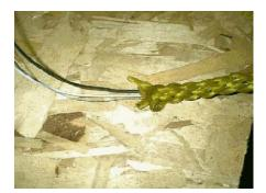
Once your head and hood are in place you will feed the wires through the center of the coreless nylon rope. To do this, grab the rope with both hands about 8" apart and compress the rope together. This will form a channel in the center that the wires will pass through. Feed the wires through the channel a few inches at a time until you have reached the end as shown in the picture to the right.
