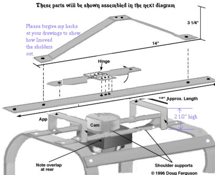
The frame shown in this step constitutes the upper body of the figure. It should be attached to a base as shown, and the base should be massive enough to support its weight such that it does not tip while in operation.
