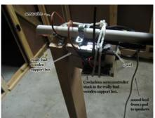
At the other end of the 5' long PVC pipe, I attached a make-shift wooden box to hold the servo controller (I bought it from <u>Cowlacious</u> rather than making it myself. I made sure the box hung down below the pipe when the skull was oriented upright. This way the skull would naturally stand straight up. Also shown in the picture is the wooden support and a metal support bracket to hold the assembly up when I am not moving the head (more on that later).
