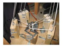
There are lots of tutorials on the Flying Crank Ghost so I am not going to go into that much detail in the mechanism itself. Here are the basics. I have a Dayton Crank motor that rotates at 6 rpm. You do need a motor with some reasonable torque o make this work. I attached a 4" wooden dowel as the shaft. I surrounded the motor with four block of wood and put 2 eyebolts in the top of each. The tendons ran through these eyebolts and to the free-rotating metal disk attached to the dowel.
