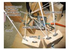
The Flying Crank Ghost (FCG) mechanism is very versatile. I use it in a different manner for <u>the crystal ball</u>. It is simply a slowly rotating shaft that pulls your strings in a way that makes your prop look alive.
