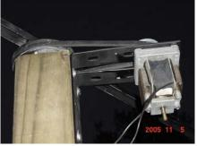
I ran a 2 1/2" lag screw down through the pulley wheel into the 4x4 (you'll have to do this BEFORE you attach the U-channel on top). I then mounted two 4" angle irons to the top back side of the 4x4 - which I used to mount my electric motor.
