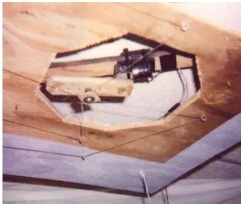
The motor's mounting beam is made of plywood, and is screwed to the large piece of plywood on plywood legs to hold it up so the crank is at the same level as the large piece of plywood.
